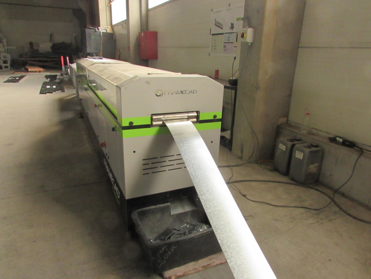
This machine produces the steel frame of a GEMINI 60 house in just 3 hours.
