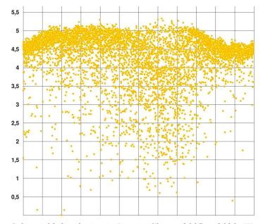
Solar yield distribution in Lawra, Ghana, 2005 to 2020. We used hourly yield estimations of 47 different locations to simulate how off-grid fast-charging settlements could reduce energy costs for transportation.
